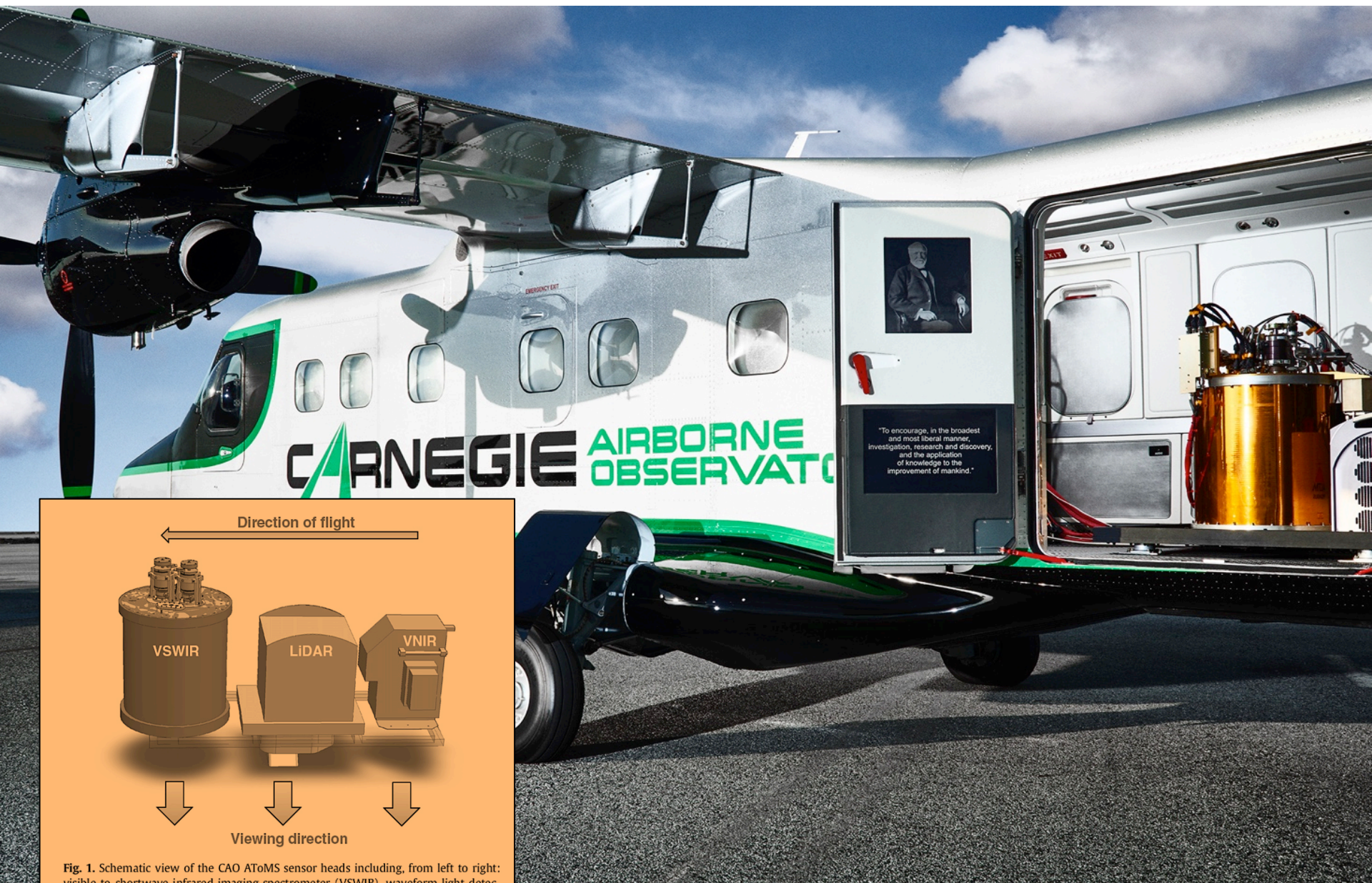
Fig. 1. Schematic view of the CAO ATOMS sensor heads including, from left to right: visible-to-shortwave infrared imaging spectrometer (VSWIR), waveform light detection and ranging (LiDAR) scanner, and visible-to-near infrared imaging spectrometer (VNIR).
